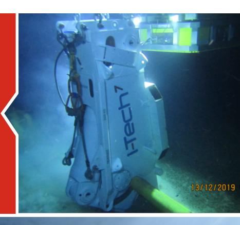
Subsea 7 Shear cutter is used for performing scrap cuts on materials up to 558mm OD (22") for example it can be used to cut various types of structures, rigid and flexible pipelines, umbilical's, tubing, H/I beams and casings. We can perform cuts using both topside control with downlines, or ROV supply using hotstabs. The shear is fitted with multiple rigging points for various horizontal and vertical cutting positions.
