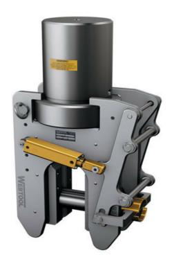
The RCV115 is a heavy duty wire rope cutter designed for subsea deployment in severe working conditions. The integrated hydraulic anvil removes the need for diver intervention and makes the tool easily deployed and operated by ROV. Corrosion resistant and durable coated steel and stainless steel construction. Genuine Webtool™ blades and anvils give optimum cutting performance and ensure that maintenance is kept to a minimum.
