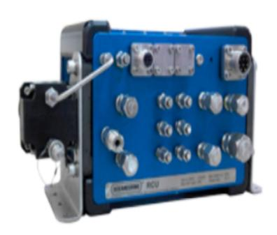
The RCU consists of two main parts, The surface unit and the Subsea unit. The surface unit consists of a laptop PC with a RS232-485 convertor providing communication interface to the subsea unit. The PC comes pre-installed software for controlling the Subsea unit. The Subsea valve module is capable of setting two different pressures, This allows separate pressure to the latch cylinders verses the torque motor on the API 17D Class 1-4 Torque Tool.
