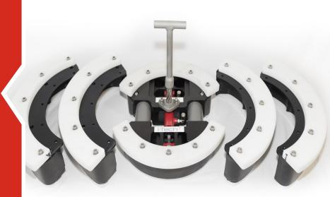
This (internal grip) Gasket Tool was designed to remove and install AX/VX gaskets (seal rings) without metal-to- metal contact between tool and sealing faces of both gasket and wellhead. With over 200 pounds of mechanical force, the Gasket Tool maintains a firm grip on the internal face of the gasket in the event of hydraulic failure. An adapter shoe system allows the tool to be configured for 13-5/8", 16-3/4" or 18-3/4" gaskets.
