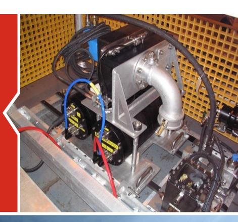
The AZ20 system is designed for the installation and blow out of suction piles. The system comprises four main components: An AnchorZip 20 suction pump; a non-invasive flow meter; a differential pressure transducer housed in a bottle; and a data acquisition bottle (to collect and record the data from the system)
