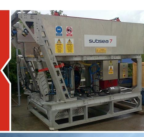
The Mock Up ROV is used for onshore integration trials to ensure all ROV serviceable areas of a subsea structure are accessible by the system.
