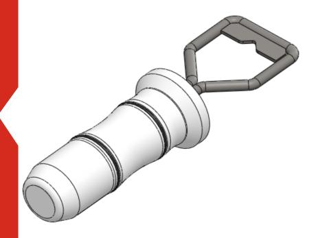
This stab is used to protect the bore of i-Tech's 3" Low Pressure Receptacle against marine growth and physical damage. Standard handle configuration D-handle with Fish Tail handle and T-handle available on request.
