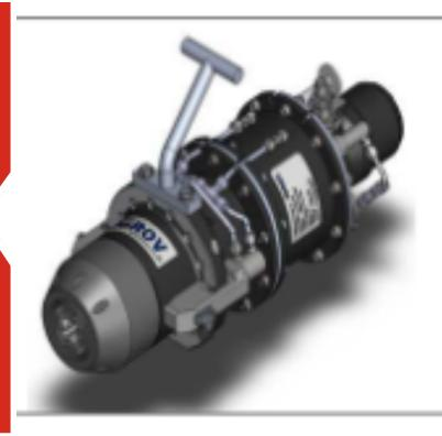
The Class 1 to 4 Torque Tool provides a means of developing torque for actuation of valves, lockdown clamps and other ancillary equipment installed as part of subsea production systems that requires actuating torques within the range of 27Nm to 2710Nm (20 to 2000 ft.lb).
