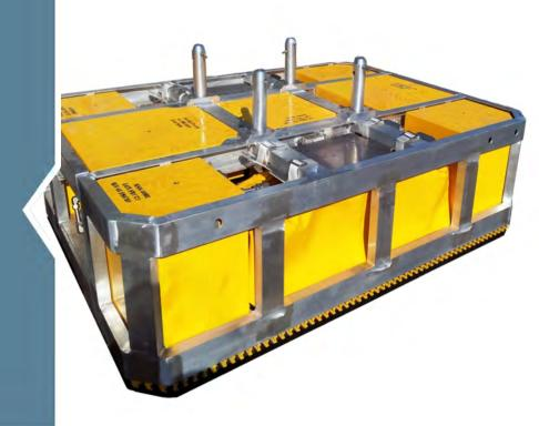
The ISP 10,000 BOP Intervention Skid is designed to provide subsea control fluid or corrosion inhibitors for BOP intervention, via a hotstab. The skid incorporates two fluid pumping circuits high flow/low pressure and low flow/high pressure to give as fast as possible closing speed under actual well conditions. The unit can be remotely switched between three pre-set outlet pressures up to a maximum of 690 bar (10,000 psi). The skid is serviceable without removal from ROV.
