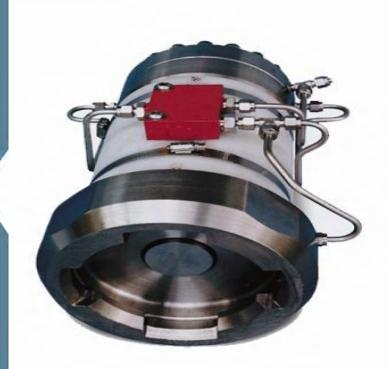
The linear actuator override tool (LAOT) is used to transmit axial force to the stem of hydraulically actuated gate valves. The tool consists of a bayonet or horse shoe profile end effector that locks the tool to the valve interface and reacts the axial override force generated by the tools piston.
