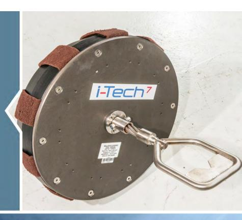
This tool was designed to remove soft growth and debris from wellhead seal interfaces for 18-3/4", 16-3/4" or 13 5/8" AX/VX gaskets (seal rings). The plastic hub prevents damage to the seal interface. Each pad is keyed in place to prevent them from slipping out of position. They are also installed individually, making pad replacement simple to perform. The top plate is ported to prevent pressure differentials while cleaning. The tool comes in a rugged weather-proof case.
