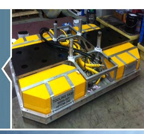
The AP Fluid Skid is designed to supply high pressure fluids subsea.
