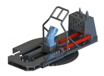
The low profile cutting tool consists of a large disc which is directly mounted to a hydraulic motor. The disc is mounted to a sliding housing which is hydraulically actuated in order to provide the correct force on the disc to allow ease of cutting. A reversible clamping mechanism is incorporated into the main body of the tool which firmly holds the tool in position during cutting.
