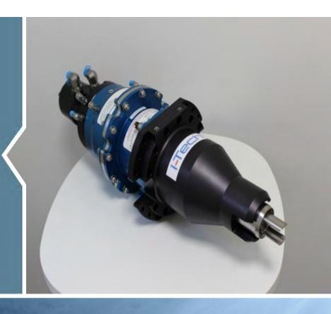
The Multi-Torque Tool provides a means of developing torque for actuation of valves and lockdown clamps, throughout a subsea production system over a torque range of 27Nm to 2710Nm (20 to 2000 ft.lb).
