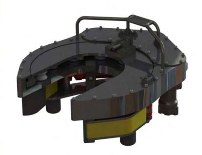
The cutting tool is designed to cut pipe ranging in size from 8" to 12" OD. The tool consists of a standard lathe parting tool which is securely mounted to an indexing head. A hydraulic motor rotates the tool around the pipe, the parting tool is indexed inward with each rotation.
