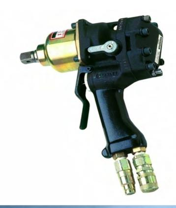
Powered by a Stanley integral Hyrevz motor, the IW12 has a durable swing hammer impact mechanism with adjustable impact intensity from 250 to 1,200 ft.lb (340 to 1,632 Nm) of torque. Designed to run from a wide range of hydraulic circuits, this wrench allows underwater bolting in the most extreme applications.
