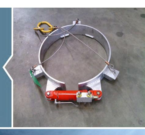
The gasket installation tool is a multi use tool that was developed to install the AX, VX-2 and the VGX-2 gaskets. It will position the gasket on the wellhead, prior to the connection procedure or re-establishment of the tree assembly. It can be used in situations where the wellhead flange has a integral tubing hanger.
