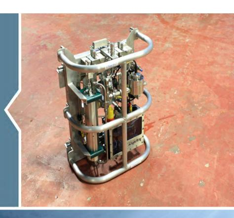
In operation this system will be used to provide glycol (Multi-Fluid) at 690 bar (10,000 psi) via a quad port hotstab (stab is not supplied with the panel). A 16 Litre (4.2 US gal) glycol compensator is supplied with the panel to provide the fluid required. The panel is also supplied with its own control system which can proportionally control the pump pressure and flow, select which of the quad ports are in use and supply feedback about supply flow, return flow and compensator volume.
