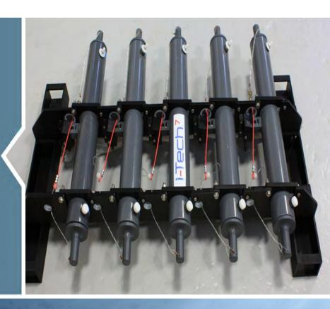
The i-Tech7 Water Sampler Kit (WSK) ITH-0029-DR-1000-00 has been designed to allow the fitment and activation of multiple (5) Nisken water sampling canisters. The cylinders are mounted to an ROV mounted frame and utilise a hydraulic drive to trigger the sample. The Canisters can be utilised to take multiple samples at the same depth or can be triggered at different depths to give comparison over the water column.
