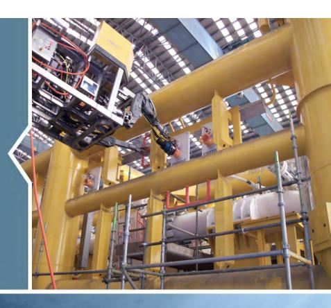
The Mock Up ROV system is used for onshore integration trials to ensure all ROV serviceable areas of a subsea structure are accessible by the system.
