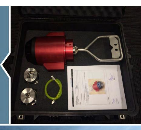
The 5:1 torque multiplier is designed to operate rotational valves on subsea structures through the use of the ROV manipulators or Torque tool. The multiplier can be used to open stuck valves as the input torque from the Torque Tool can be closely monitored so the output torque does not exceed the breaking torque of the valve.
