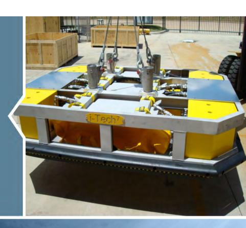
The (Automatic Selective Flow<sup>™</sup>) ASF<sup>™</sup> Fluid Skid is designed to provide subsea control fluid or corrosion inhibitors for BOP intervention, via a hotstab. The skid incorporates two pumps to give both high flow and high closing pressure. The pumping system automatically switches between pumps, allowing the system to optimise the flow and pressure requirements to suit the BOP. The ASF<sup>™</sup> can be used for regular BOP tests or emergency closure.
