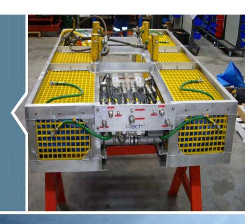
This skid is designed to provide high flow/high pressure fluid that will allow the BOP Blind Shear Rams (BSR's) to meet the stipulated closure time laid out in API Std53. The skid utilises a triple pump configuration to provide high flow and high pressure fluid when required. The BOP fluid is delivered by high pressure lines to a 17H high flow hotstab. The total fluid carrying capacity of the skid is 700 L (184 US gal).
