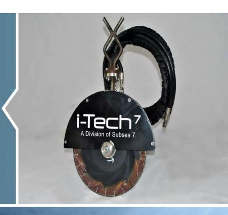
The super cutter is a versatile cutting tool that is manipulated by the ROV. The diamond encrusted blade is interchangeable with carbide tooth blades depending on the material being cut. The tool has a cutting depth of 114mm. The motor drives the blade via a pressure compensated bearing housing to ensure maximum life and protection for the drive motor.
