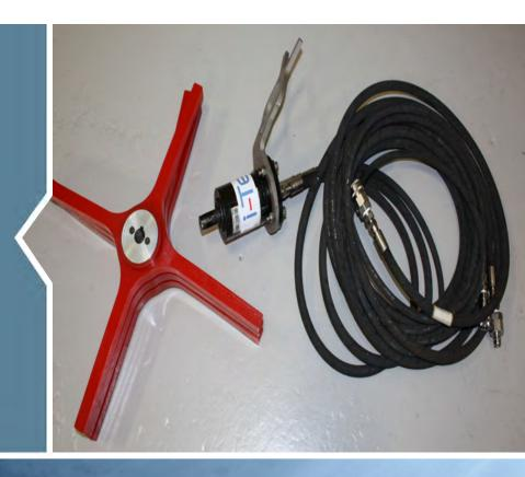
The removal tool is designed to remove marine growth from tubular subsea sections. It attaches directly to the 5 function manipulator to improve the tools cleaning capability. The tool consists of two hydraulically driven contra rotating cleaning discs which, when fitted with appropriate flails or abrasive material will effectively remove marine growth.
