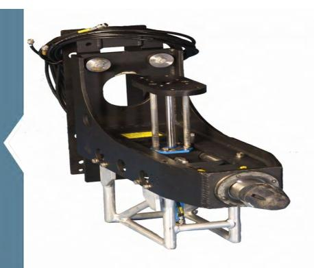
The single point tool deployment unit (TDU) is used to locate and stabilise the ROV during subsea intervention tasks. Using either standard or purpose-built tooling, the tool is light-weight and simple to interface with most work-class ROVs.
