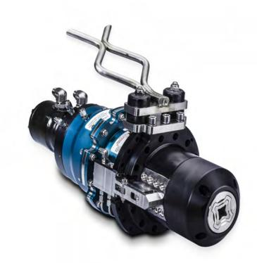
The Class 1 to 4 Rotary Docking Torque Tool provides a means of developing torque for actuation of valves and lockdown clamps, throughout a subsea production system over a torque range of 27Nm to 2710Nm (20 to 2000 ft.lb).
