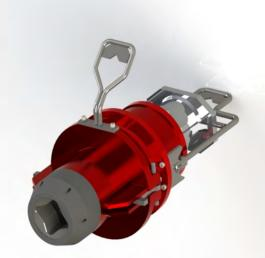
The class 4 to 7 toque tool adaptor is designed to handle class 7 valves and connectors through a standard class 4 torque tool. The adaptor is pressure compensated and has a mechanical latch mechanism activated through the vertical grab handle.
