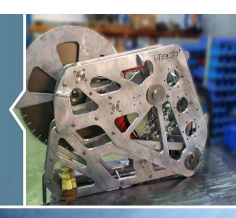
The Diamond Disc Cuting tool consists of a large disc which is directly mounted to a hydraulic motor. The disc is mounted on an arm which is hydraulically actuated and provides the correct force on the disc to allow ease of cutting. A clamping mechanism is incorporated which firmly holds the tool in position during cutting.
