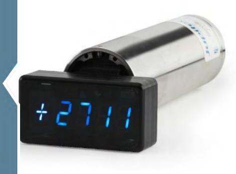
The turns counter is designed to display the total number of sensor actuations on subsea tools, modules and installations without the need for a complex control system or data link which allows a critical cyclic operations to be monitored at low cost. The turns counter can be set to count every actuator pulse at rates up to 10 pulses per second. The turns counter allows full quadrature up/down counting.
