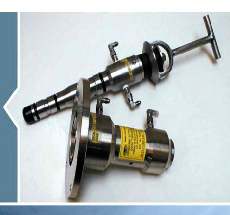
Our dual port hot stab and receptacle conform to both ISO/API 17H and ISO 13628-8 Type A specifications. The hot stab's body is made of strong Nitronic 60 for longevity. The nose can be in bronze or nylon and replaced if it becomes damaged, yet it cannot be spun off accidentally. The standard handle for hot stab is a T-handle. D-style and fishtails are also available. Various seal configurations can be offered to suit specific operations.
