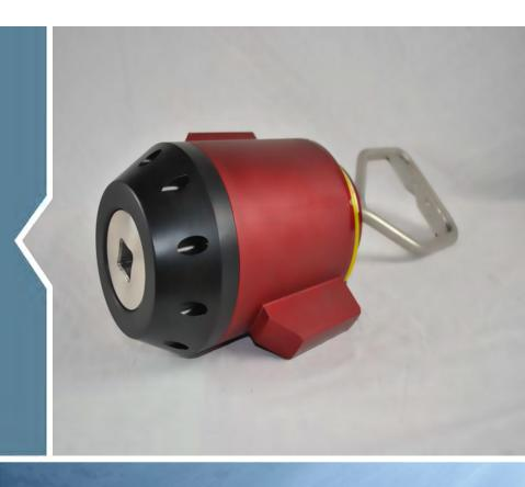
The 3:1 Torque Multiplier is designed to operate rotational valves on subsea structures through the use of an ROV. The tool provides a 3:1 torque multiplication ratio by which the torque is transmitted from the manipulator wrist of the ROV through to the end effector. The end effector shown is suited for ISO 13628:8 Class 1 & amp; 2 interfaces. Other end effectors can be fitted if required.
