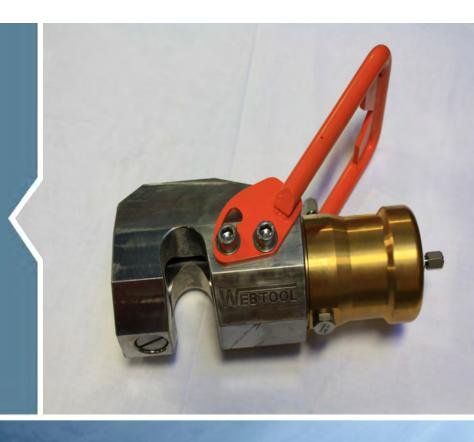
The 38mm (1.5") wire rope cutter is an ROV deployed tool which is used to cut 1770N/mm² grade wire rope of up to 38mm diameter.
