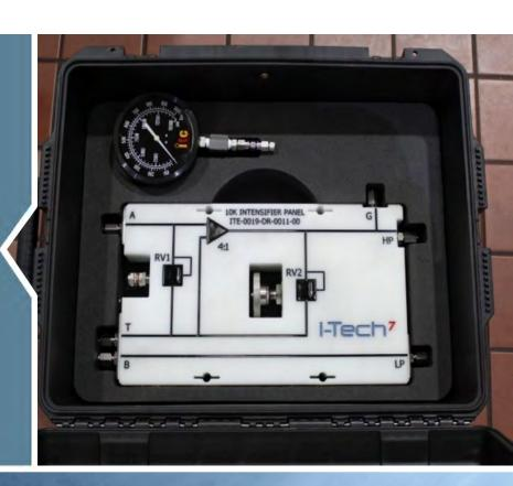
The hydraulic intensifier panel is a compact lightweight unit designed to fit easily to a host ROV used in conjunction with an intervention tooling system where high pressures hydraulics are required.
