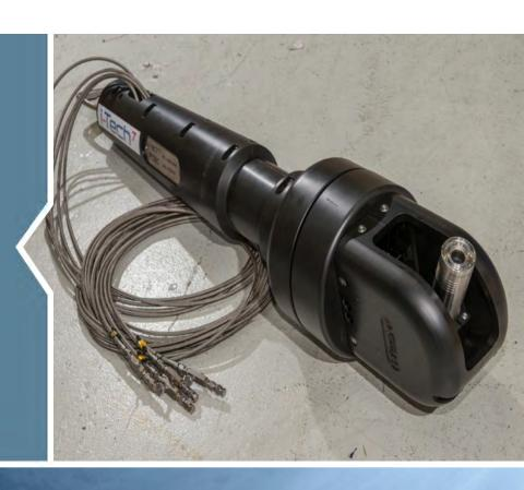
The P.T.Z.I.C. offers a complete subsea viewing package. The camera utilises an ROV hydraulic pan and tilt unit providing 200° pan and 78° tilt movement. The zoom camera is a stainless steel unit with integrated LED lights and RS232 control.
