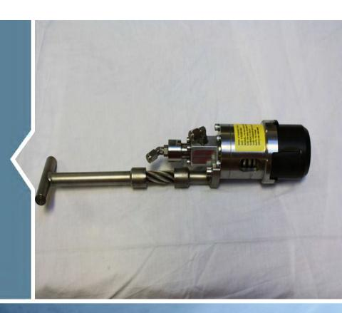
This Gasket Tool was designed to remove and install 3" (75mm) AX gaskets (seal rings) without metal-to- metal contact between the tool and the gasket. The Gasket Tool maintains a firm grip on the gasket in the event of hydraulic failure. The bolt-on T-handle shown is included as standard. Option handles such as fish tail (ITH-0012-DR-1300-00) and D (ITH-0012-DR-1400-00) handles are also available.
