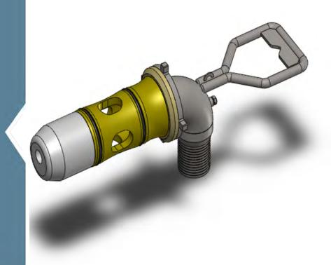
This hot stab is typically used as the pumping tool for suction piles. It has a Delrin nose on the front end of the assembly which registers in the receptacle to reduce wear and impact damage to the stab's aluminium anodized body. This assembly comes 1/4 " port for installation of transducer or gauge sense line at the stab. The fitting is a 3" hose barb nipple for convenient hose attachment. Standard handle configuration D-handle with Fish Tail handle and T-handle available on request.
