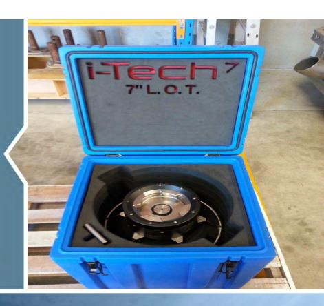
The Hydraulic Release Variable Stroke Lock Out Tool connects to the front of a Type A Linear Actuator Override Tool and is used to lock Linear Valves. Once locked the LAOT can return to the surface or be used on another valve.
