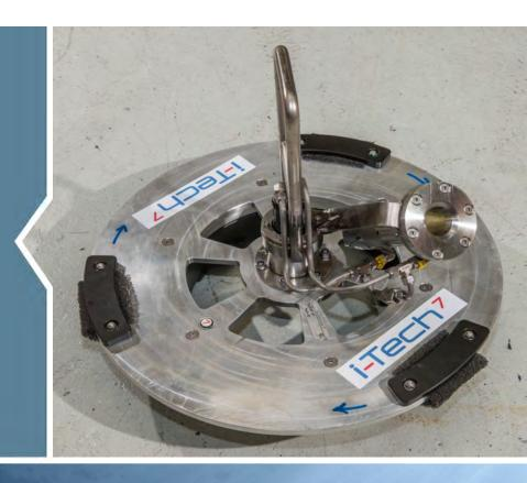
The Wellhead Cleaning Tool has been designed to remove any residual gasket coating or oxidised scale from the conical VX sealing face of a wellhead prior to the connection process or re-establishing of the tree assembly.
