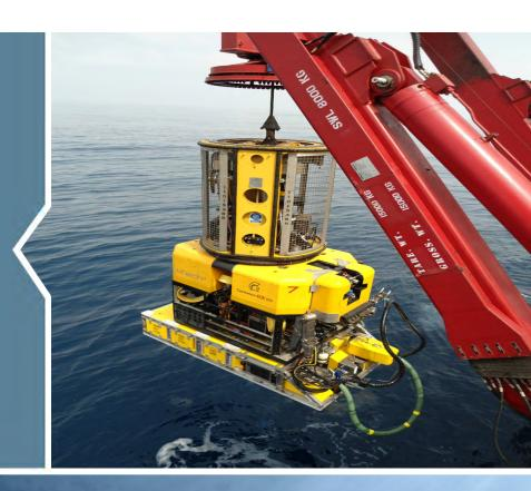
The Subsea Hydrocarbon Sampling Skid is Subsea 7 patented technology designed to hot stab into flowlines to allow Mono-phasic hydrocarbon sampling from live production wells for flow assurance, PVT and GOR studies. Production fluid chemistry analysis of oil condensate, formation water enabling Calibration of subsea flow metersFiscal allocations.
