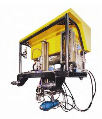
Deployed from a workclass ROV, the tool deployment unit (TDU) ensures a safe and efficient intervention operation. Using two docking probes, rather than attaching with a grabber or suction pad, the system is able to locate and stabilise the ROV in a known position and precisely deploy a dedicated tool via an XYZ mechanism.
