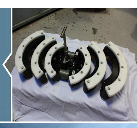
This Gasket Tool was designed to remove and install AX/VX gaskets (seal rings) without metal-to-metal contact between the tool and the gasket. With over 200 pounds of mechanical force, the Gasket Tool maintains a firm grip on the gasket in the event of hydraulic failure. An adapter shoe system allows the tool to be configured for any gasket size between 13-5/8" and 18-3/4".
