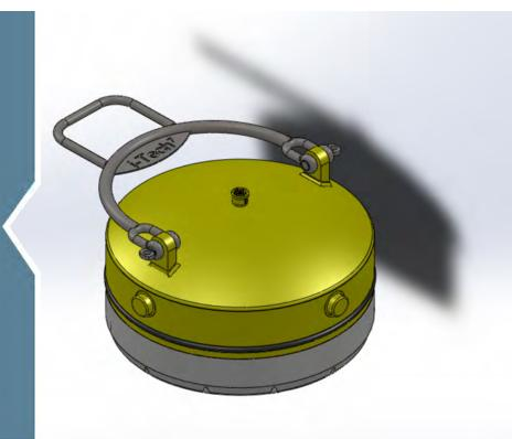
Suction pile plugs are part of our suction pile installation/retrieval suite of tools and components. In addition to plugs, i-Tech offers the mating receptacles and parking receptacles. This system replaces butterfly valves and is available in a variety of sizes. This plug can be easily removed and recovered by the ROV for seal replacement.
